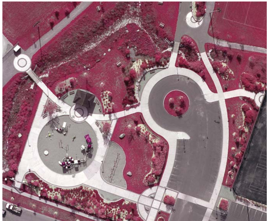
6in GSD CIR image from an Applanix 39 Megapixel DSS aerial camera.
